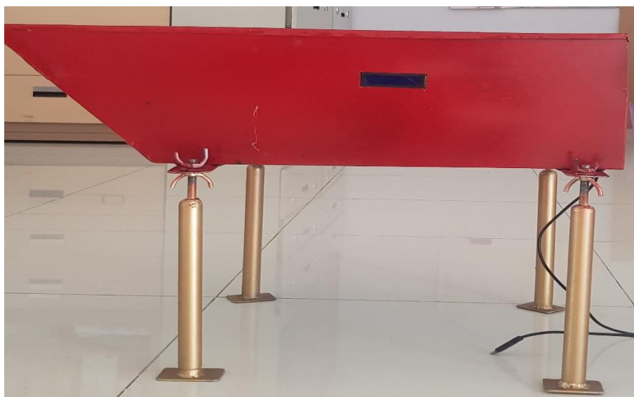
Figure 7. Mockup Precision Approach Path Indicator
