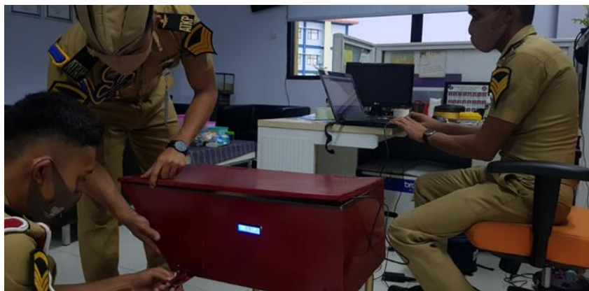
Figure 14. The precision calibration exercise of approach path indicator (PAPI)
